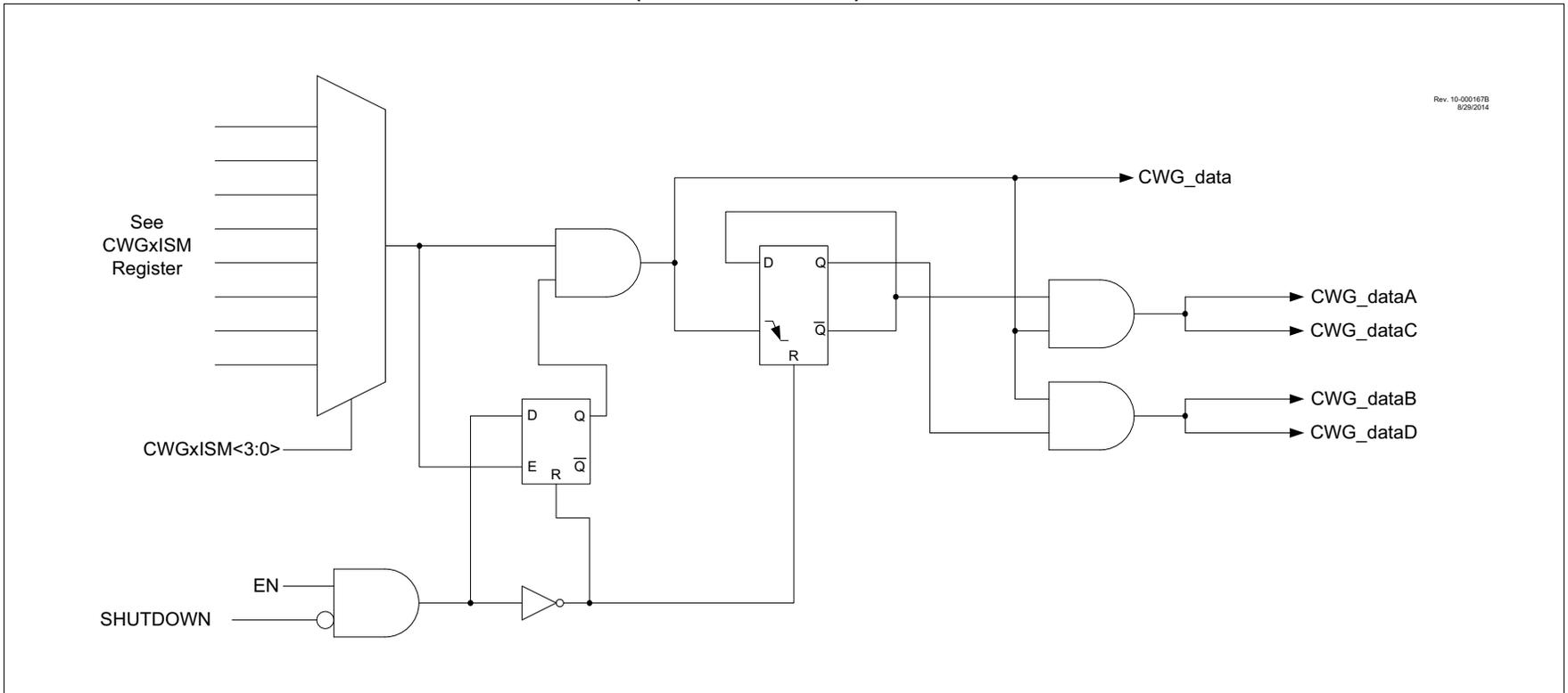
FIGURE 20-3: SIMPLIFIED CWG BLOCK DIAGRAM (FORWARD AND REVERSE FULL-BRIDGE MODES)
