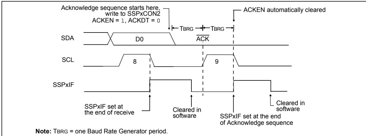
**FIGURE 31-31: STOP CONDITION RECEIVE OR TRANSMIT MODE**
