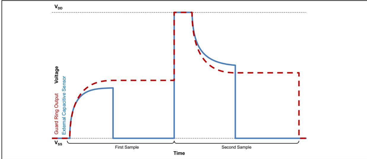
**FIGURE 23-10: HARDWARE CVD SEQUENCE TIMING DIAGRAM**
