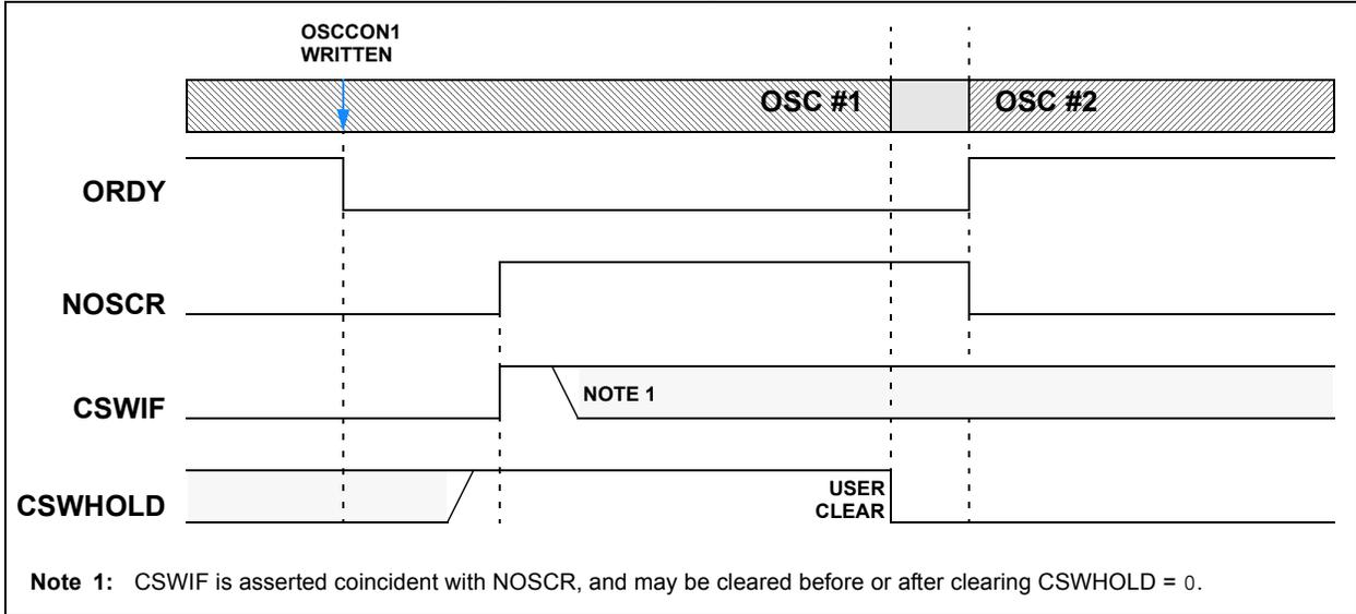
**FIGURE 6-8: CLOCK SWITCH ABANDONED**
