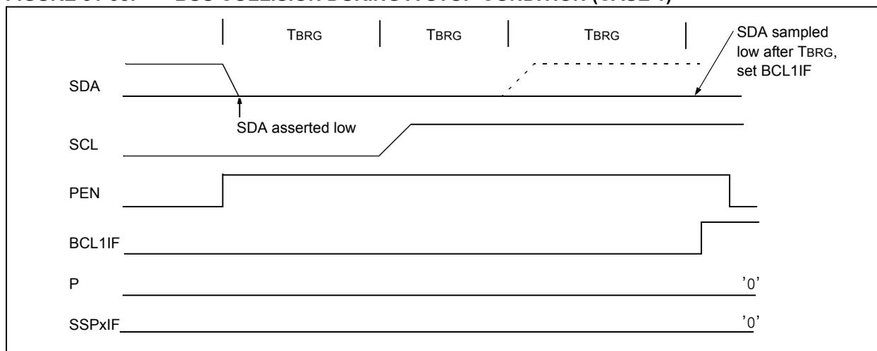
**FIGURE 31-39: BUS COLLISION DURING A STOP CONDITION (CASE 2)**
