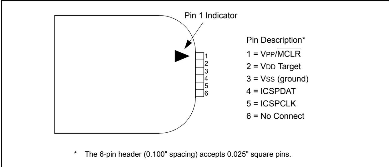
**FIGURE 35-3: TYPICAL CONNECTION FOR ICSP™ PROGRAMMING**
