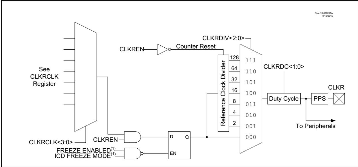
**FIGURE 34-2: CLOCK REFERENCE TIMING**
