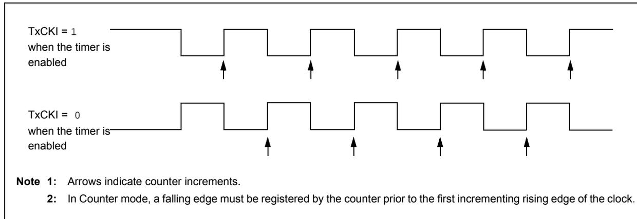
**FIGURE 28-3: TIMER1 GATE ENABLE MODE**
