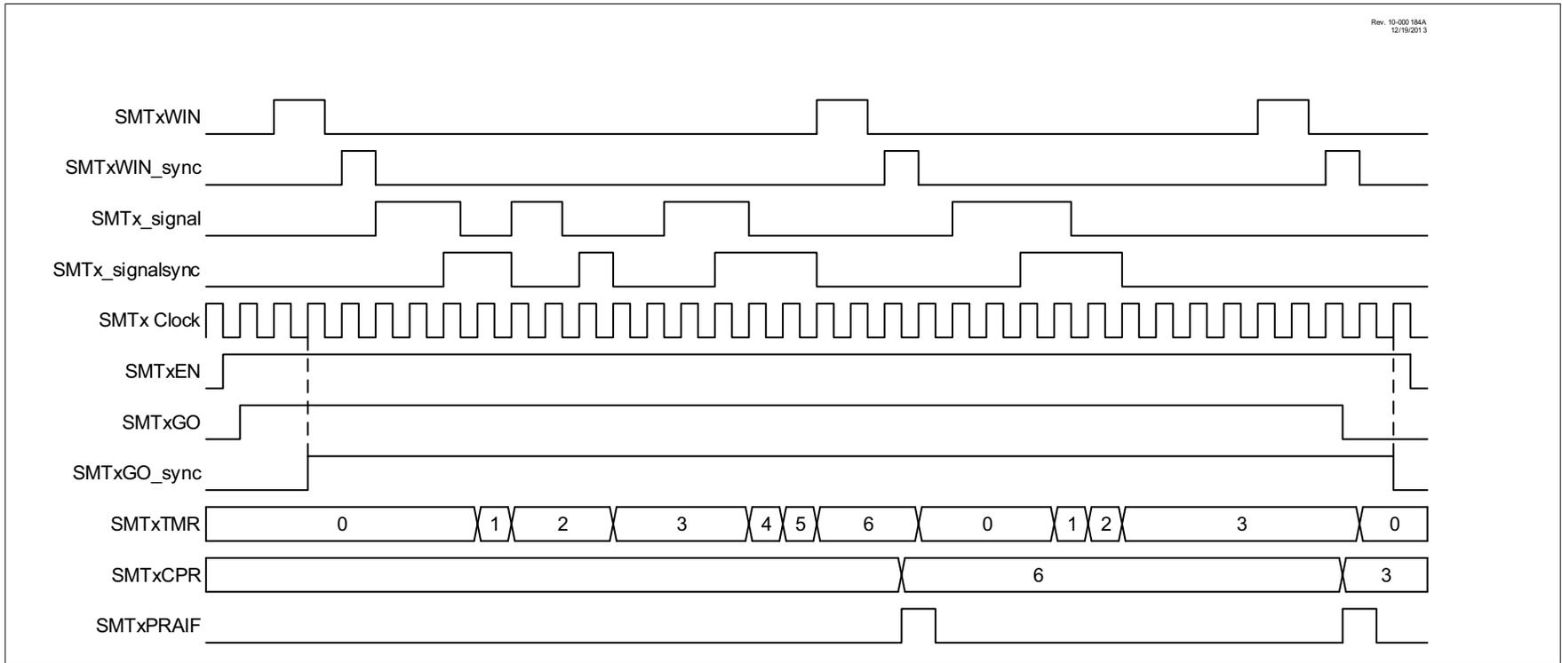
**FIGURE 32-13: GATED WINDOWED MEASURE MODE SINGLE ACQUISITION TIMING DIAGRAMS**
