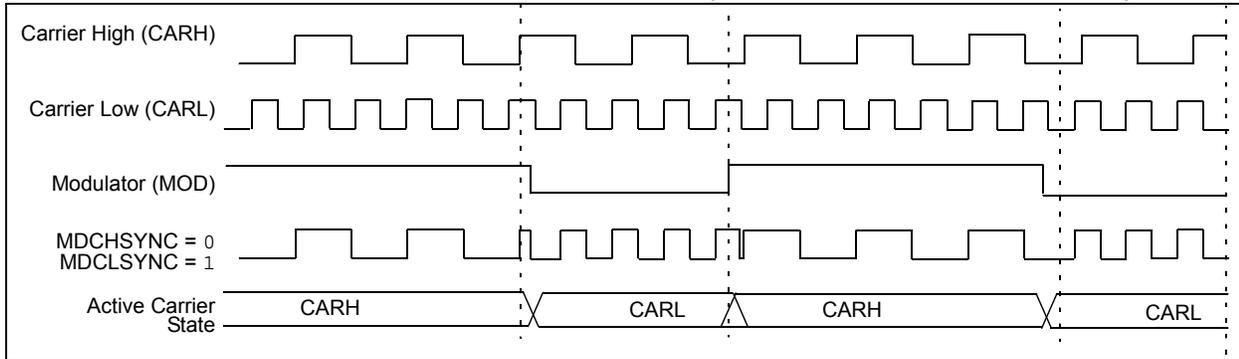
**FIGURE 26-6: FULL SYNCHRONIZATION (MDSHSYNC = 1, MDCLSYNC = 1)**
