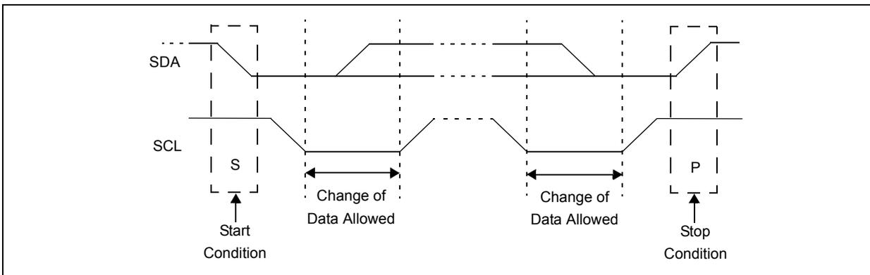
FIGURE 31-13: I<sup>2</sup>C RESTART CONDITION
