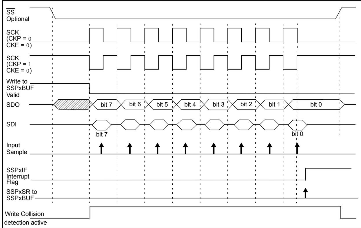
**FIGURE 31-10: SPI MODE WAVEFORM (SLAVE MODE WITH CKE = 1)**
