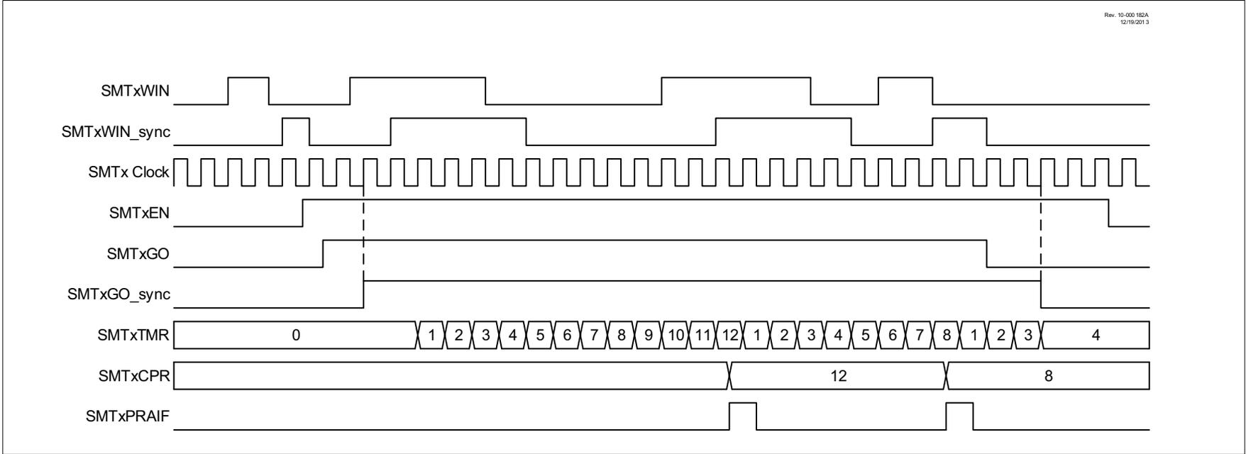
**FIGURE 32-11: WINDOWED MEASURE MODE SINGLE ACQUISITION TIMING DIAGRAM**
