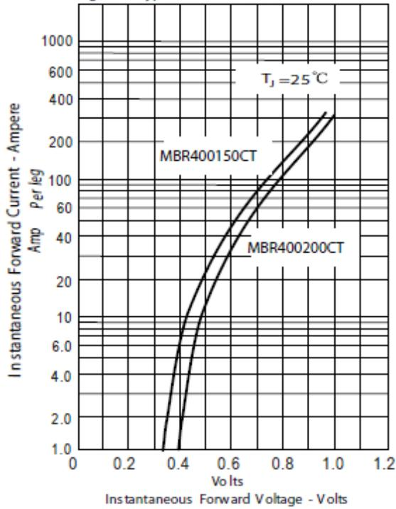
Figure .2- Forward Derating Curve
